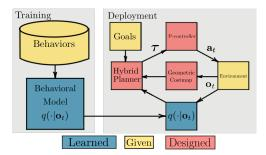
**Fig. 3: HIP system diagram:** A dataset of trajectory demonstrations is used to learn a model of traversability and behavior. The model is combined with a geometric costmap into the hybrid planner, which plans a trajectory towards a received goal.
