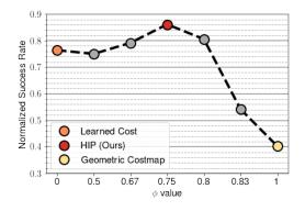
Fig. 7: Success rate on varying  $\phi$ : When no cost is incorporated ( $\phi = 0$ ), our method purely relies on learning; when the learned component is removed ( $\phi = 1$ ), our method purely relies on the costmap. Empirically analyzing a range of  $\phi$  suggests that combining the components with  $\phi = 0.75$  results in the best performing system.
